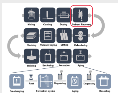
Schematic LIB manufacturing process
