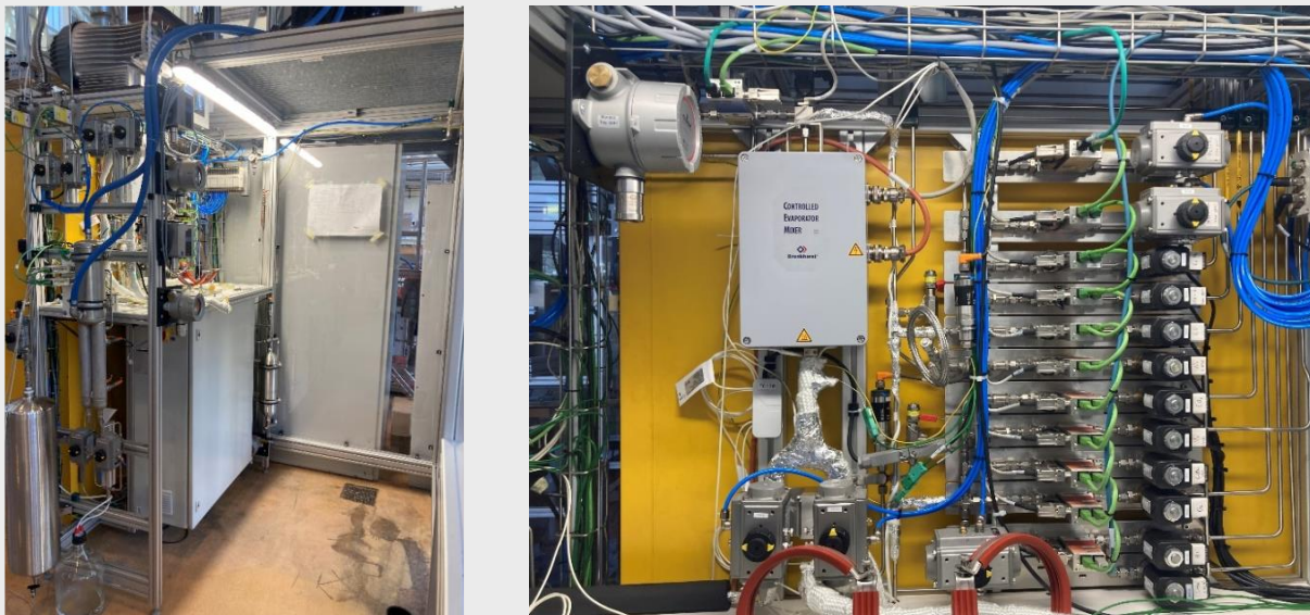
Typical experimental setup used for membrane testing with gases containing impurities.
