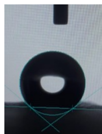
Contact angle measurement of a hydrophobized Flexiramic surface of 142 °
