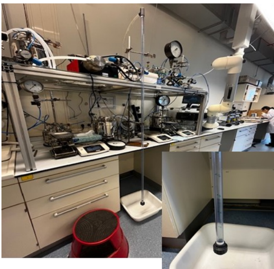
Set up to measure burst pressure
