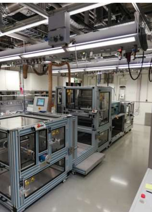
Figure 7. PL7 Roll-to-Roll Coating of Advanced Nanophase-Segregated Ion-Exchange Polymer Membranes
