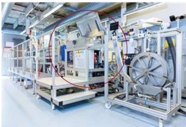
Figure 10. PL10 In-line modification of nanocoatings on polymeric HF's (University of Twente)
