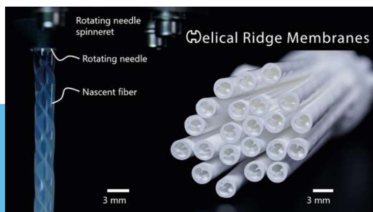
Figure 13. PL13 Hollow fiber membrane spinning with improved geometric features (RWTH)
