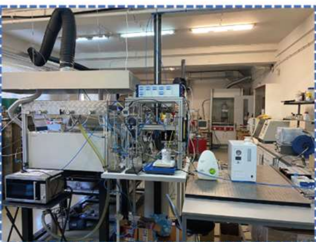
Figure 12. PL12 Up-scaled CVD/ALD deposition unit for the tailoring of the nanopore size of ceramic and stainless steel Molecular Sieving membranes (DEMOK)
