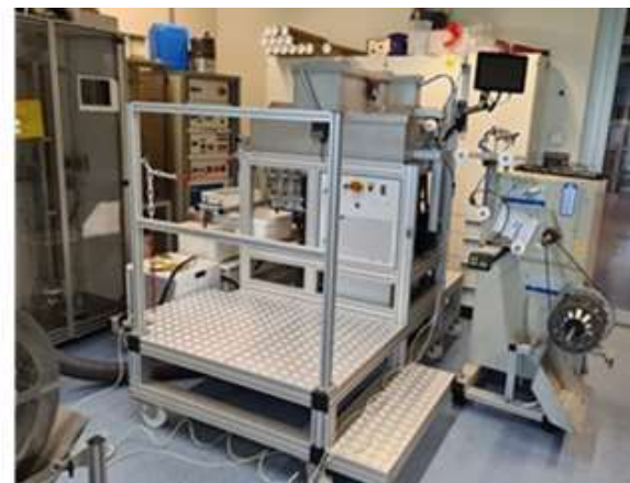
Figure 10. PL10 In-line modification of nanocoatings on polymeric HF's (University of Twente)
