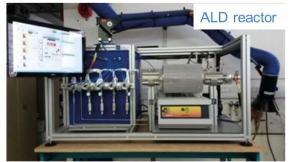
Figure 8. PL8 Surface modification of polymeric hollow fibers by co-co-extrusion or Atomic layer Deposition (ALD)
