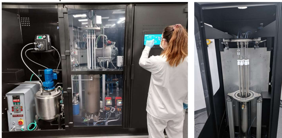
Figure 1. Membrane manufacturing pilot plant (left) and non-destructive permeation properties setup (right).
