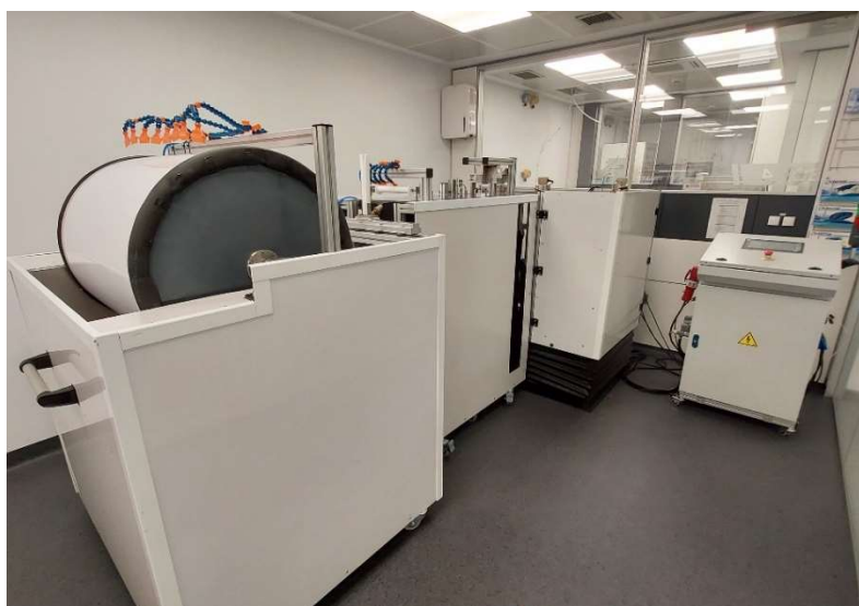
Figure 1. Up-graded dual layer mixed matrix membrane spinning line at Tecnalia
